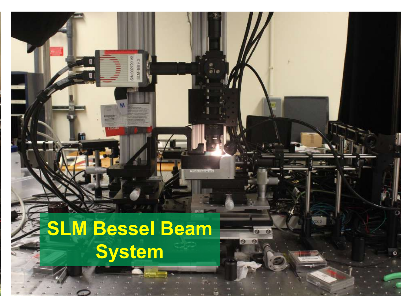
Fig. 3 SLM-Bessel Beam System enables high precision rapid z-scanning in four dimensions, allowing observation of active neural dynamics in the nerve ring of C. elegans .
