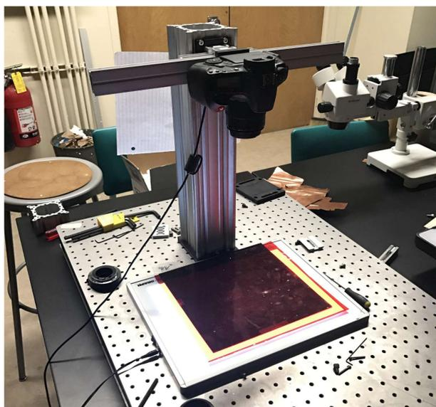
**Above:** Microscope setup with Canon 60-D camera and filtered light. Control QW1217 worms with regular dietary levels are traced in agar plates, then behavior is tracked and compared to that of L-serine treated worms using Worm Tracker.
