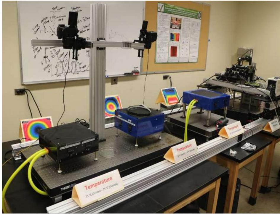
Microscope setup in which the microscope can slide and move from one experiment to the next to facilitate worm tracking. The microscope can take data from the various temperature plates around to take temperature experiment data.
