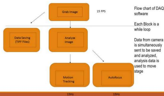
Algorithm used to do worm tracking, We take an image, then use the image data to move the stages in order to accurately track the worm.
