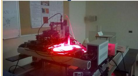
Microscope setup over a temperature plate. This is a linear gradient that can be anywhere from 0.2 C/cm to 0.6 C/cm, to study behavior such as isothermal tracking.
