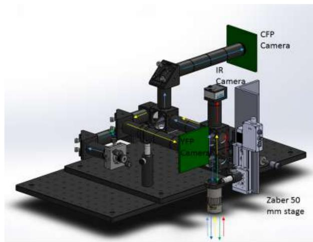
Side view of the worm tracking microscope with labeled parts.
