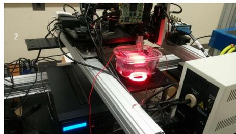
Microscope setup over an electric field experiment. This experiment involves subjecting worms to electric fields from 4-12 V/cm
